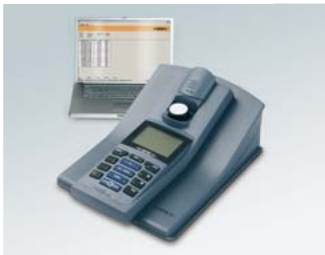
NEW: A turbidity measuring lab for in the field – the new Turb 430IR/T sets
